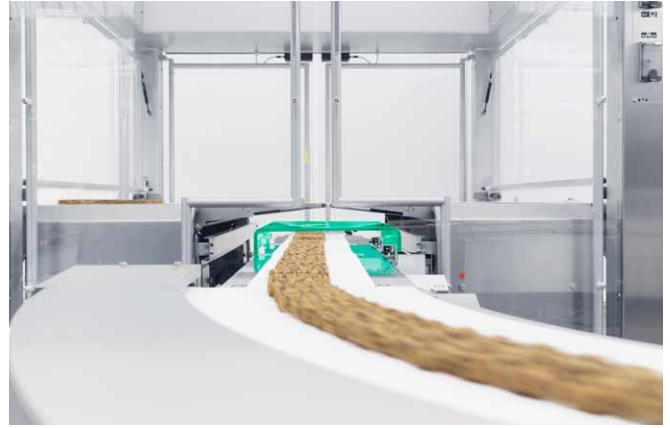
The product rows are taken over seamlessly and distributed to the packaging machines.
