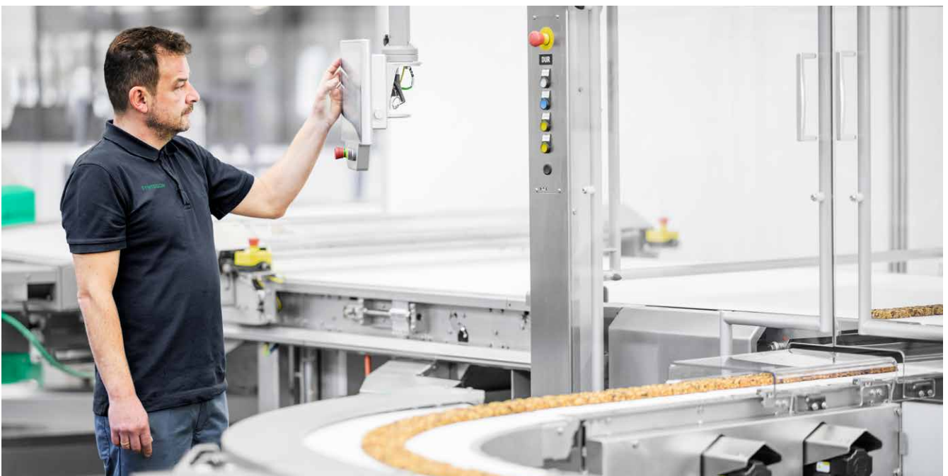
Using the HMI, operators can switch between different product and format recipes.
