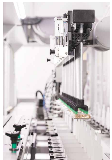
After primary packaging, the wrapped bars are seamlessly packed into folding cartons.
